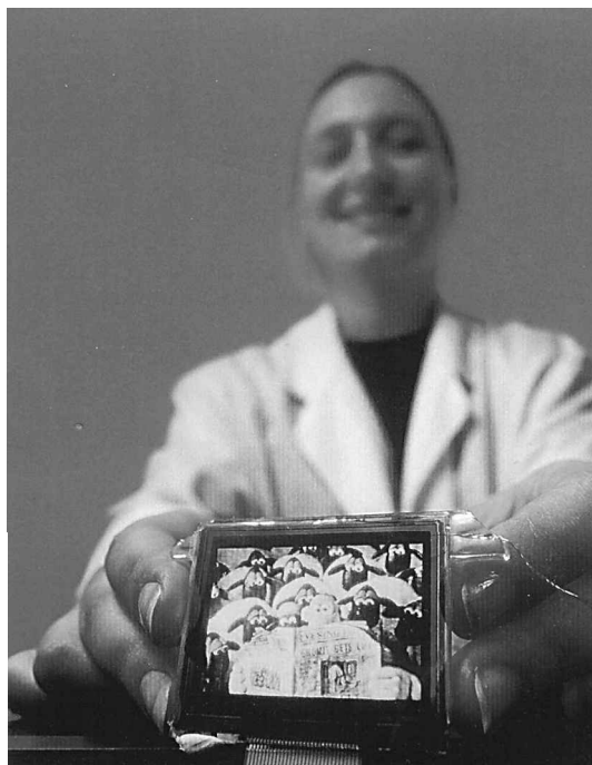
Figure 8. EL polymer graphic display prototype (courtesy of Cambridge Display Technology Ltd and of Physics World June 1999, p. 35.).
